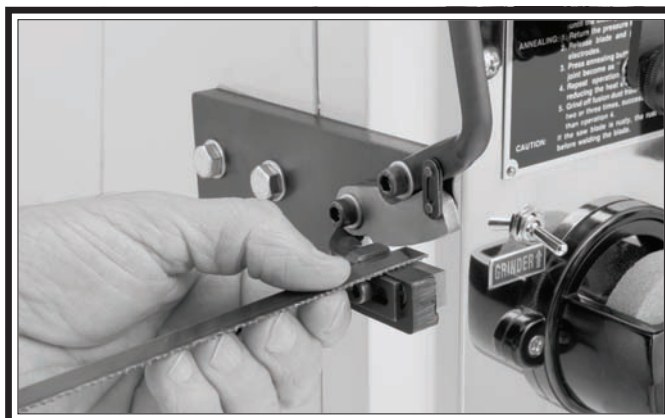
Figure 28. Using the blade shear to cut the blade.
